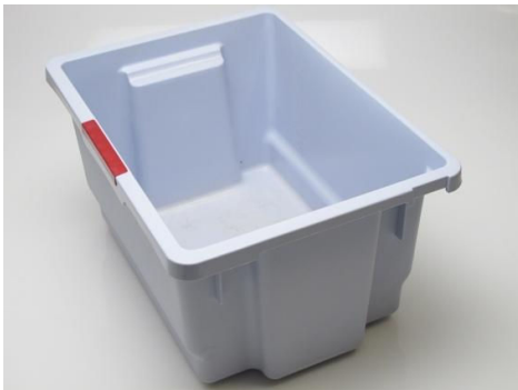
Photo: Pre-box after 80 autoclaving cycles
